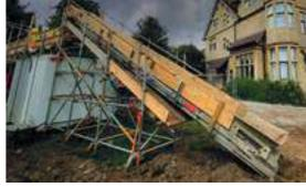
The Easikit 600™ can be used across a range of sites including large excavation projects due to its considerable output and ease of loading by machine.
